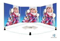
IPS displays use an advanced technology which gives you extra wide viewing angles of 178/178 degree, making it possible to view the display from almost any angle. Unlike standard TN panels, IPS displays gives you remarkably crisp images with vivid colors, making it ideal not only for Photos, movies and web browsing, but also for professional applications which
